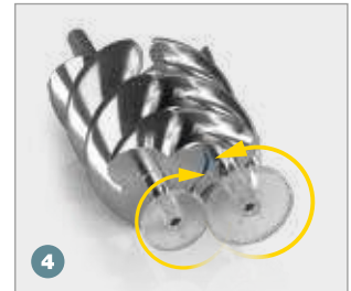
4 Flow chamber completely evacuated
